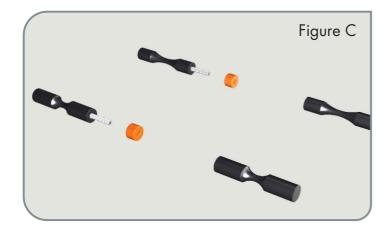
or Champagne bottles and require one (1) Magnum Spacer to be inserted between each Starter and Extension Pin (Figure C).\*\*
